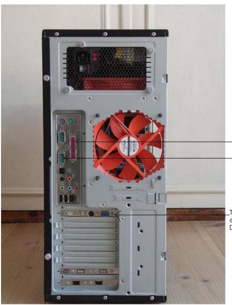
This is a Parallel Port and Tserial port where One can connect the Token - Machine.
