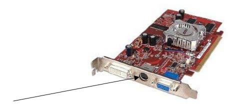
The card will have one VGA output, One S-video Output and One DVI Output
